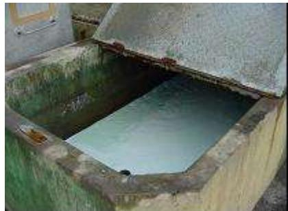
Preparation. The product (powder) is weighed and mixed in an intermediate tank. It will then be pumped into a pipe feeding the gun (pressurized pipe).
